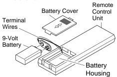
Figure 16 - Installing Battery In Hand-Held Remote control Unit
